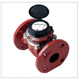
RUBIN hot water meters operate according to the flowrate measuring principle using a Woltman turbine and are designed for high-volume water measurement. The complete modular system covers a wide measuring range in all areas of water supply management or as flow meter or flow sensor for energy measurement systems.
