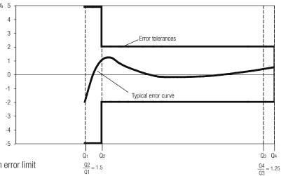
Operation error limit = 2 x calibration error limit
